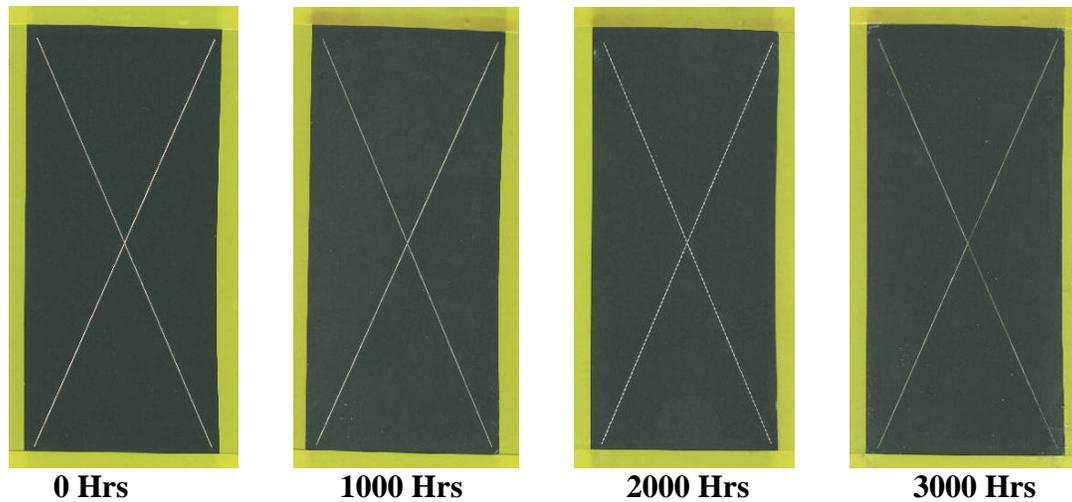
**Figure 5. Corrosion Protection Of 2024-T3 Aluminum Alloy In ASTM B-117 Salt Fog Testing**
