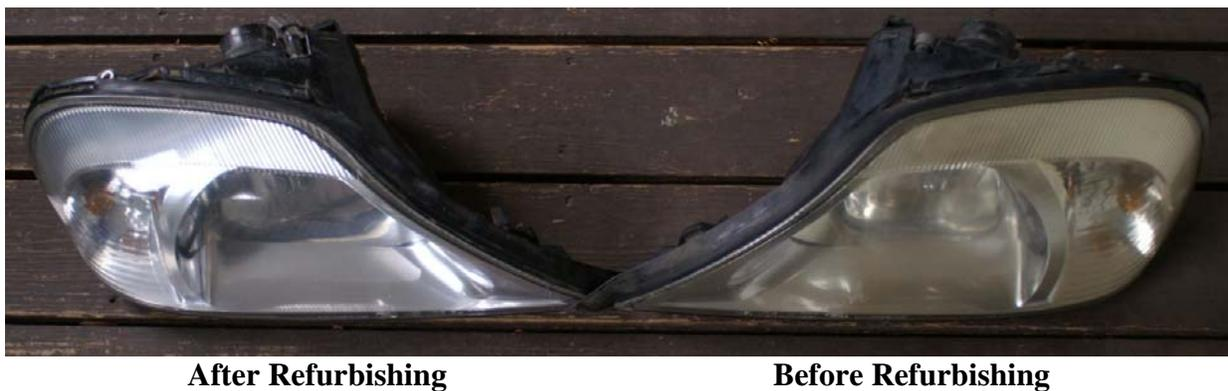
**Figure 1. Refurbishing Of Automobile Headlamp With High Performance UV Technology**
