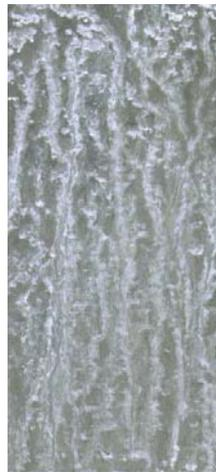
**Figure 6. 24 Hour Corrosion Of Unprotected 2024-T3 Aluminum Alloy In ASTM B-117 Salt Fog**
