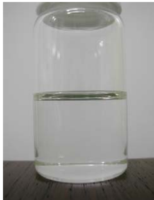
Figure 2. Example of 25wt% CSP dispersed in acrylate monomer (IBOA)
