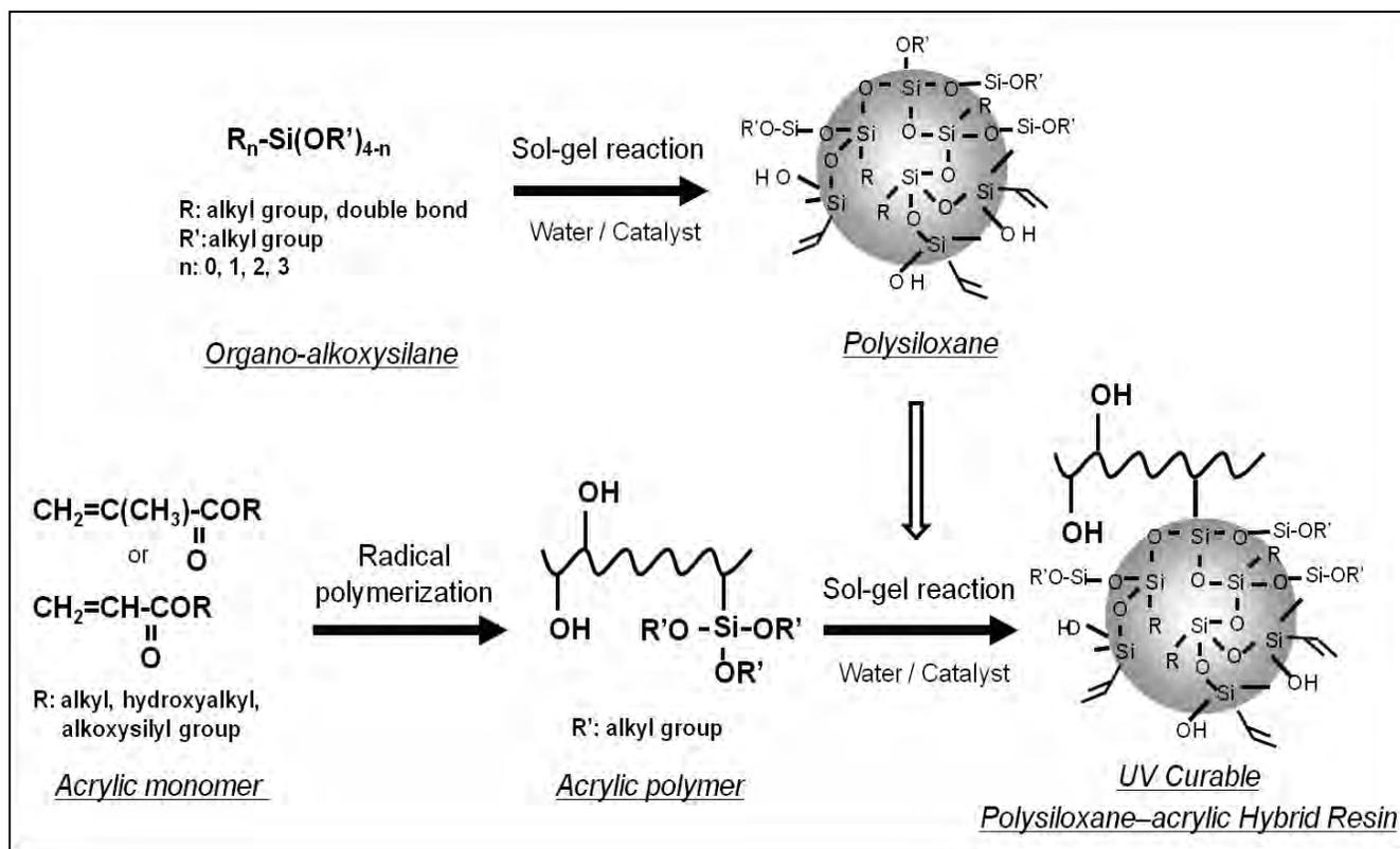
Fig.1 Hybridization of acrylic polymer and polysiloxane.
