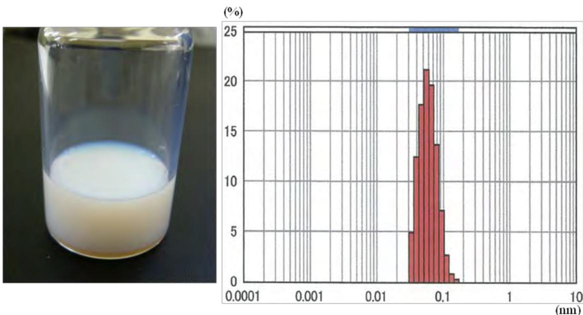
Fig.7 Appearance of the dispersion and particle size distribution.
