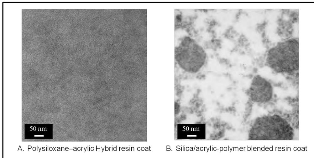
Fig.3 Film morphology of the clear coating measured by TEM
