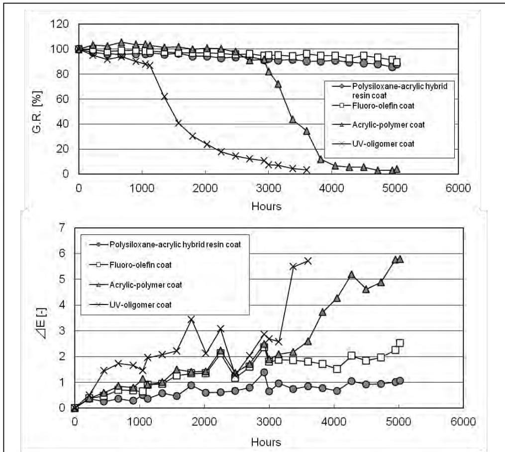
Fig.4 60-degree gloss retention and  $\Delta E$  in sunshine weather-o-meter test
