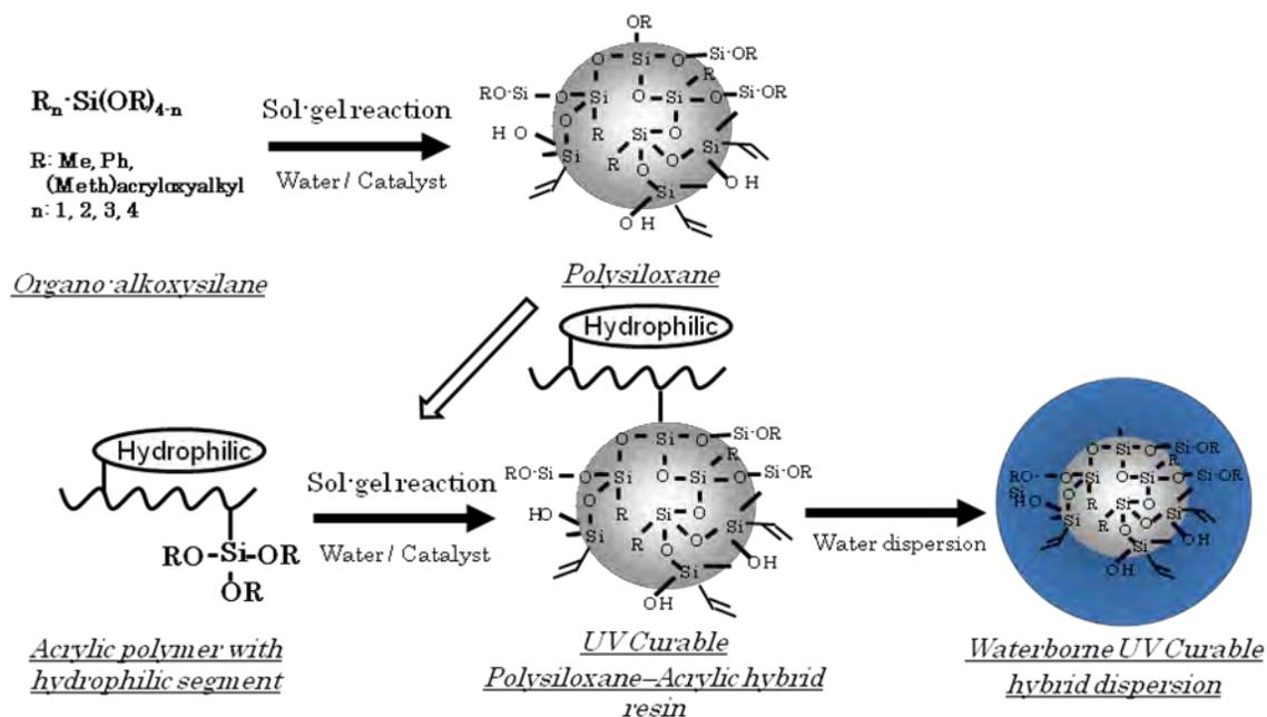
Fig.6 Waterborne UV curable hybrid dispersion
