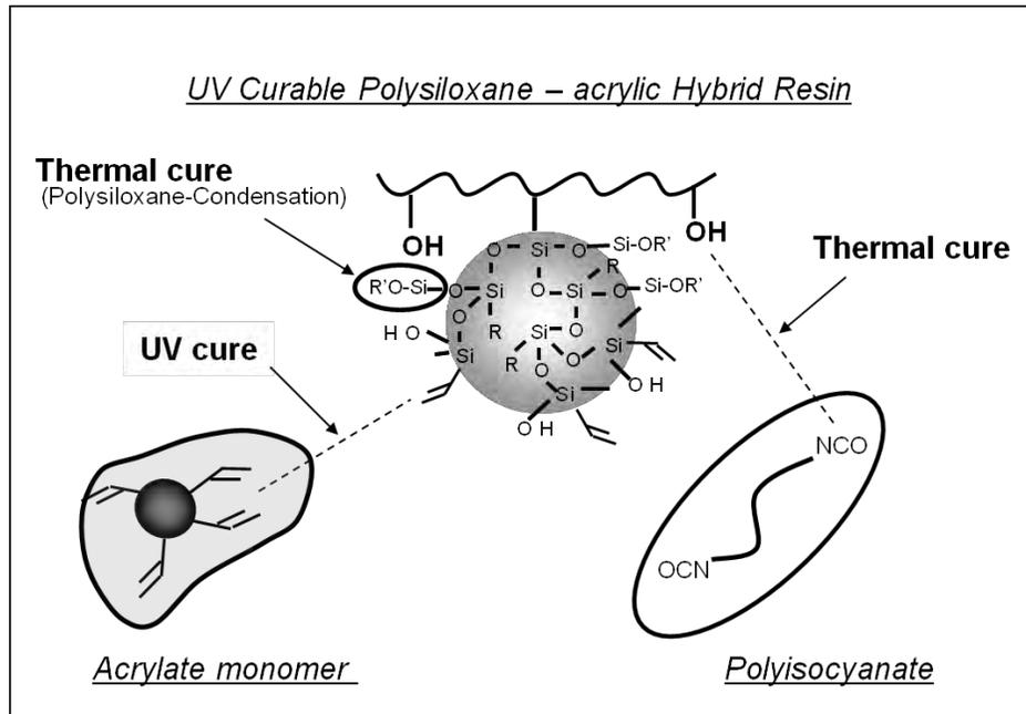
Fig.2 Cross-linking system of the hybrid resin coating
