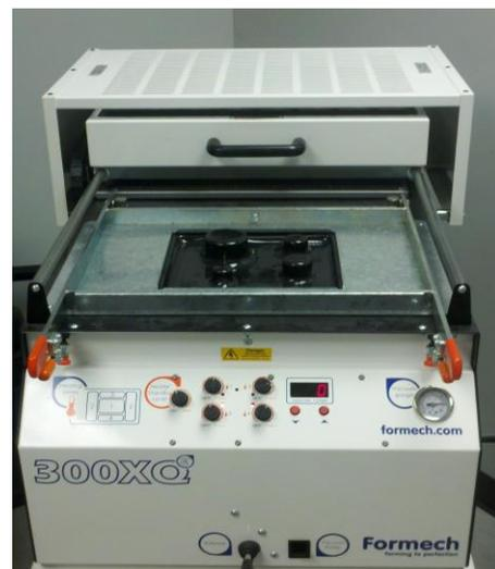
**Figure 2.** Formech vacuum forming apparatus
