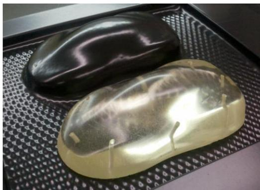
Figure 5. Complex mold used to rate degree of forming
