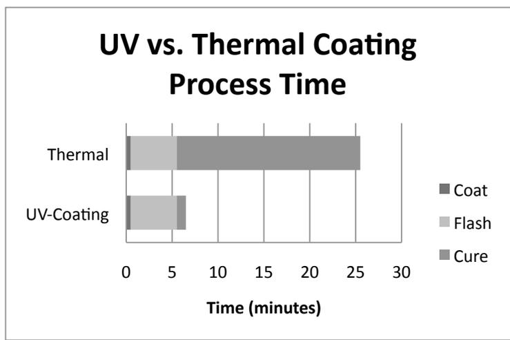
Figure 1. Comparison of general processing times for UV and thermal cure coatings
