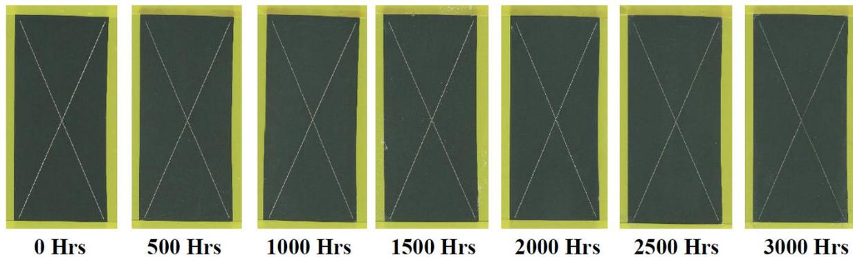
**Figure 3.** Corrosion Protection Of 2024-T3 Aluminum Alloy In ASTM B-117 Salt Fog Testing
