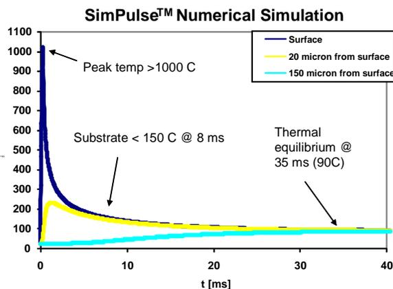
Figure 2. Thermal simulation of the photonic curing process ( $300 \mu\text{s}$ ,  $1 \text{ J}/\text{cm}^2$ ) for a 1 micron thick silver film on 150 micron thick PET. Temperatures beyond  $1000 \text{ }^\circ\text{C}$  can be achieved on PET without damage.
