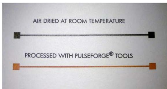
Figure 3: Image of screen-printed copper oxide reduction ink before and after conversion to copper in open air on Paper. Note the pronounced color change after processing.
