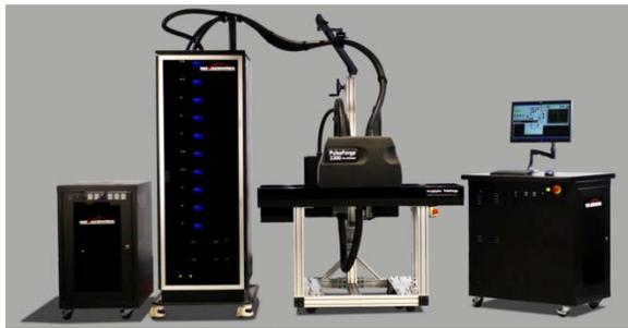
Figure 1. PulseForge® 3300 photonic curing system
