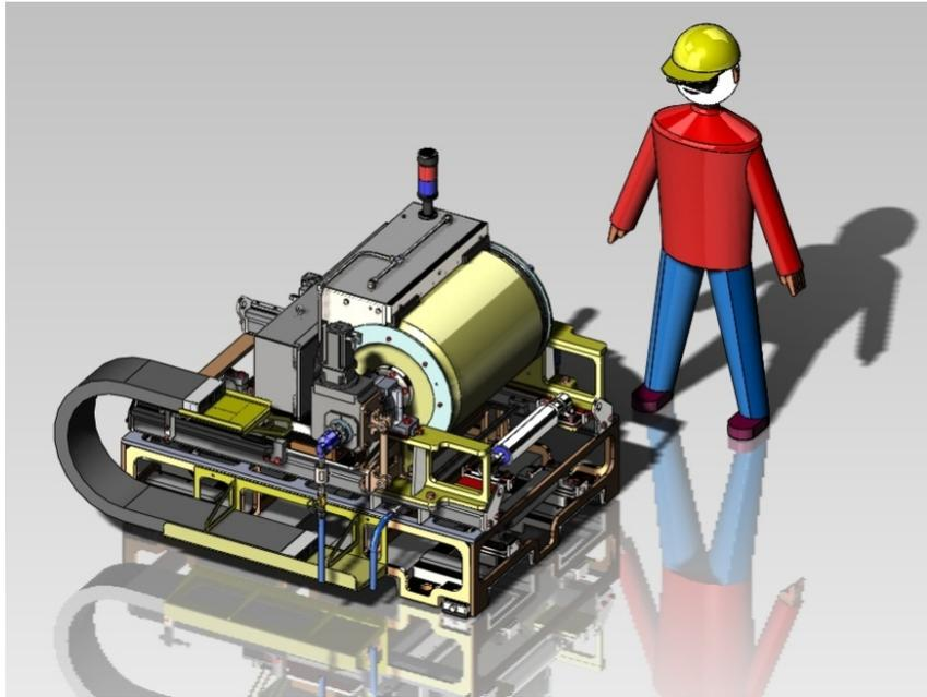
**Figure 7.** Narrow web EB system with sealed tube emitter and integrated shield roll.
