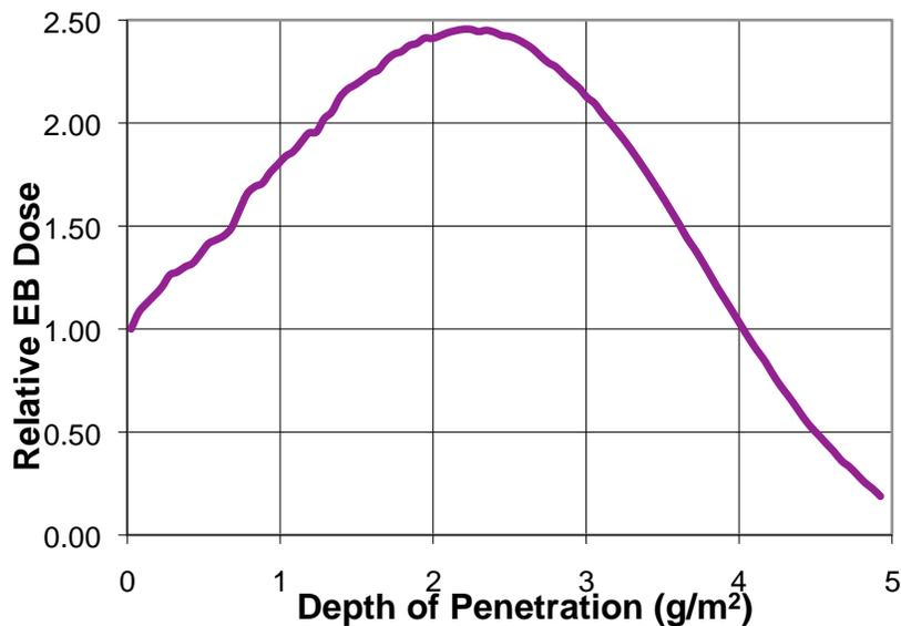
**Figure 2.** Depth/dose curve for 15 kV EB operated in  $10^{-5}$  torr.
