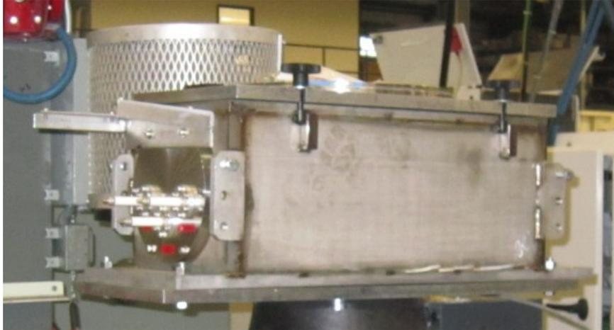
**Figure 1.** Ultra-Low energy electron beam for vacuum applications (electron gun within vacuum test fixture).
