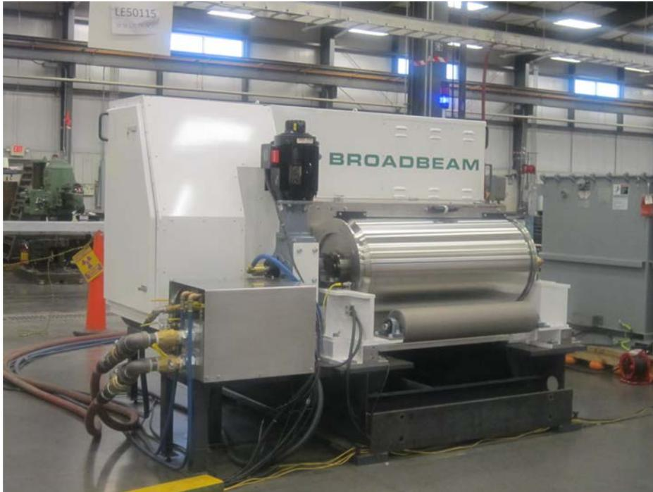
**Figure 5.** Extended voltage (175 kV) electron beam equipment.
