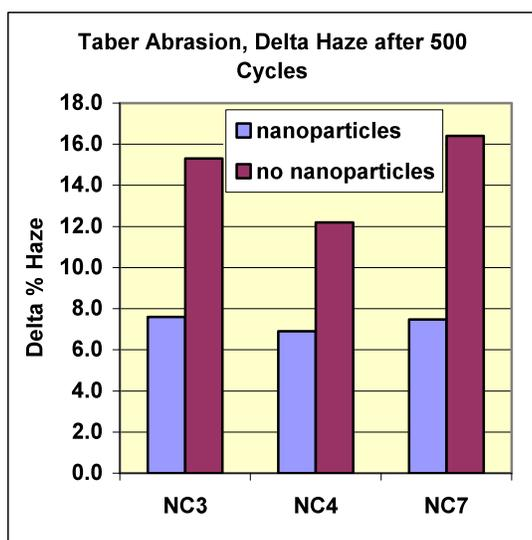
**Figure 9.** Coatings with Nanoparticles have less abrasion after Taber testing. Note: Test data. Actual results may vary.
