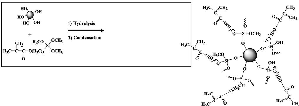
**Figure 8.** Silica nanoparticles functionalized with acrylated silane can act as reactive filler to improve properties of weatherable hardcoats.
