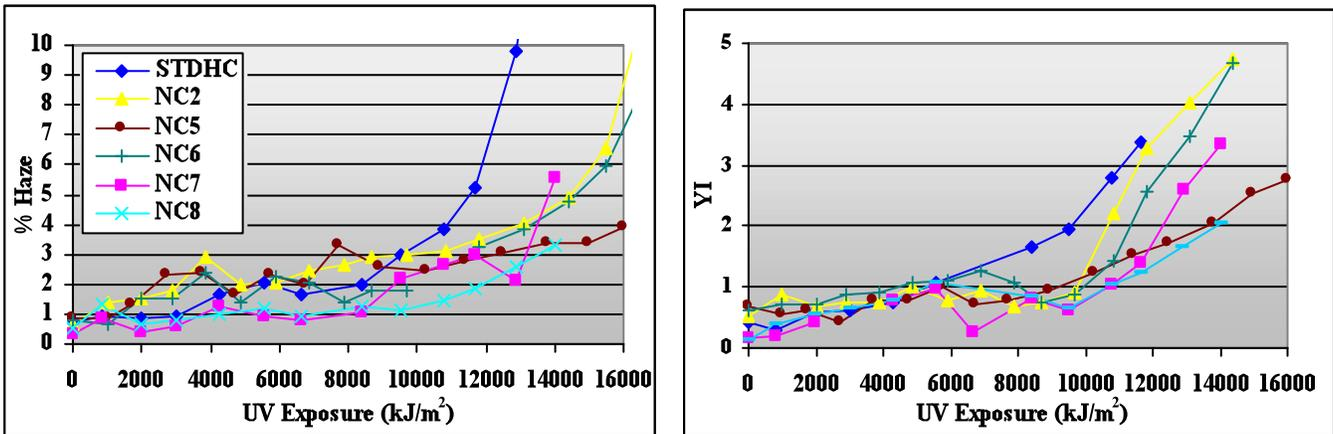
**Figure 5.** % Haze and Yellowness (YI) after Xenon Gmod weathering for some coatings with improved crack resistance compared to three-year standard formula STDHC. After 14,000 kJ/m², all of the new coatings passed the specification of % haze <7. Coatings NC5, NC7, and NC8 pass the specification of having YI<4. Note: Test data. Actual results may vary.
