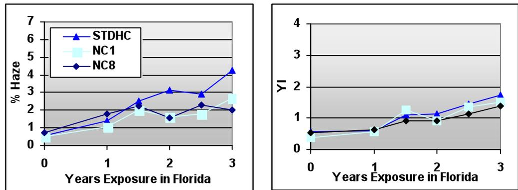
**Figure 6.** Outdoor weathering results for standard three-year weatherable coating STDHC and for new coatings NC1 and NC8 as of February 2012. All coatings showed good results after three years, as expected. Note: Test data. Actual results may vary.
