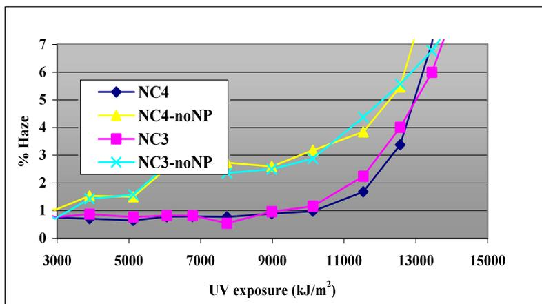
**Figure 10.** Haze after weathering for formulas NC3 and NC4 with nanoparticles and NC3-noNP, NC4-noNP without nanoparticles. Note: Test data. Actual results may vary.
