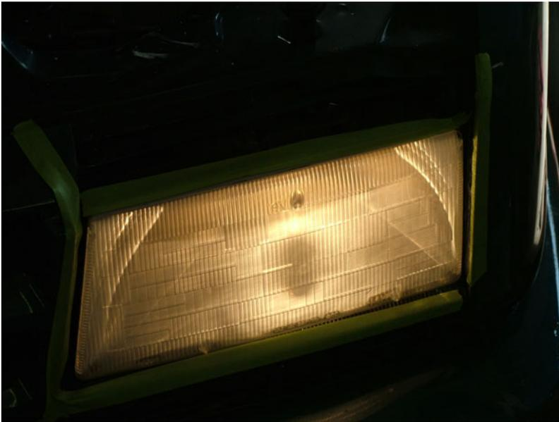
**Figure 2: Automotive Headlight with Degraded UV Cure Hard Coat**
