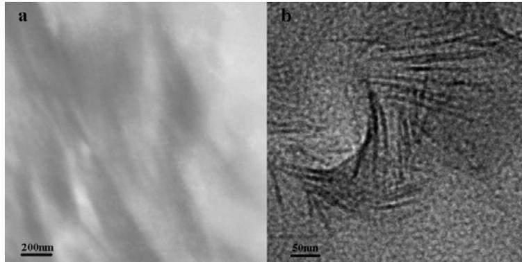
Fig. 8. TEM and HR-TEM micrographs of UV cured polymer/LDH nanocomposites at 5 wt% LDH loading.
