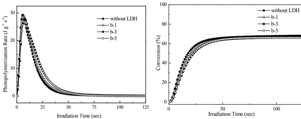
Fig. 5. Photopolymerization rates and unsaturation conversion of series B formulations.
