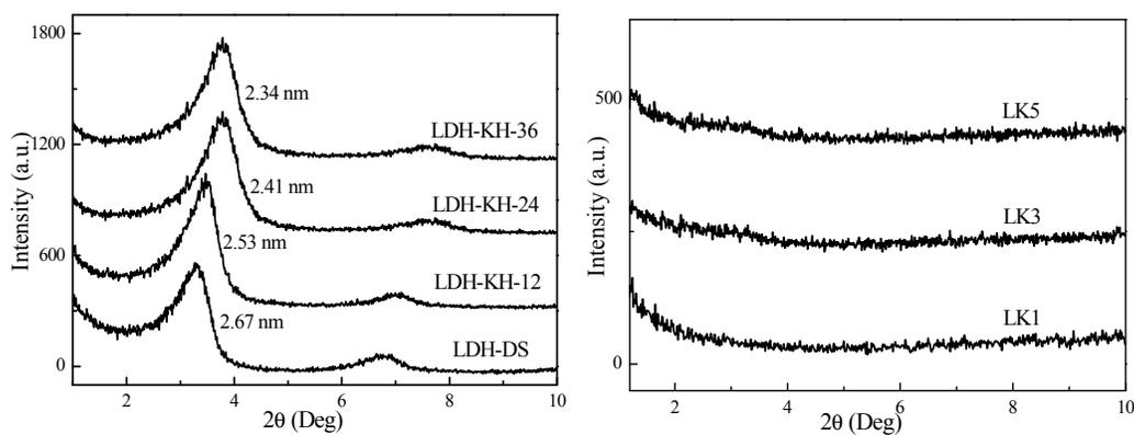
Fig. 2. XRD patterns of LDH-DS, LDH-KH, and UV cured polymer/LDH nanocomposites.
