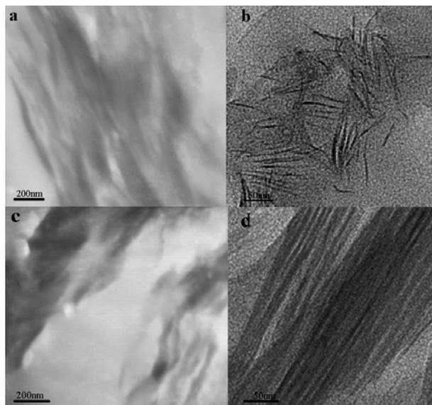
Fig. 7. TEM and HR-TEM micrographs of UV cured nanocomposites at 5 wt% LDH-1173 loading for a-5 (a, b) and b-5 (c, d).
