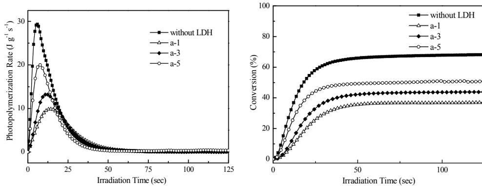
Fig. 4. Photopolymerization rates and unsaturation conversion of series A formulations.
