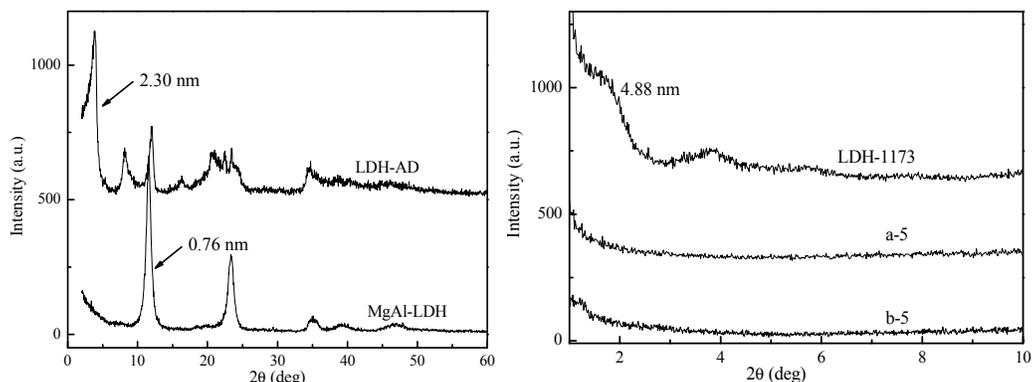
Fig. 1. XRD patterns of MgAl-LDH, LDH-AD, LDH-1173 and UV cured polymer/LDH nanocomposites.
