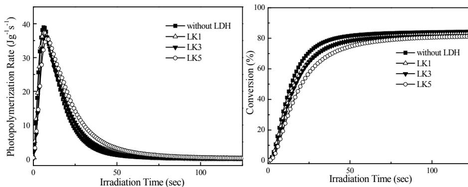
Fig. 6. Photopolymerization rates and unsaturation conversion of the LDH-KH formulations.
