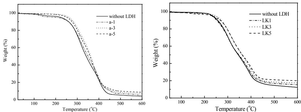
Fig. 9. TGA curves of UV cured polymer and nanocomposites with LDH-1173 and LDH-KH under  $N_2$  flow.
