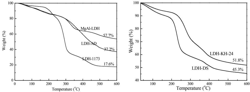
Fig. 3. TGA curves of MgAl-LDH, LDH-AD, LDH-1173, LDH-DK-24 and LDH-DK-24.
