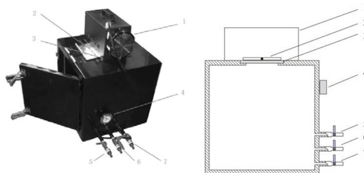
Fig. 1. Structure of the vacuum UV curing device
