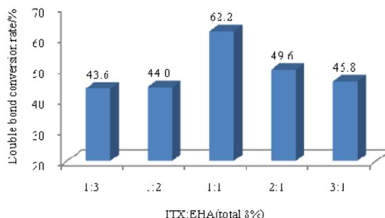
Fig.4. ITX/EHA ratio on the double bond conversion rate of UV-curable flexo ink
