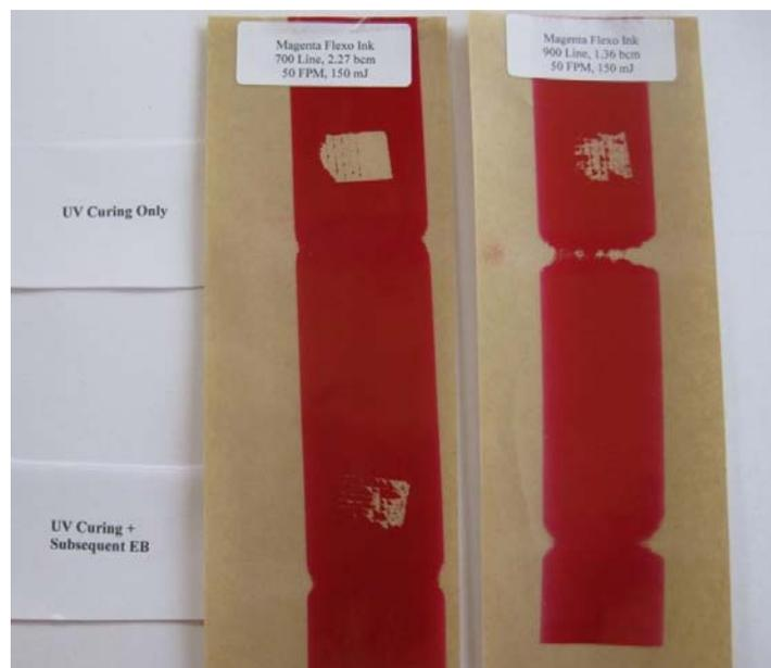
**Figure 4.** Magenta ink samples UV cured at 150  $\text{mJ}/\text{cm}^2$  at two different application weights (700 lpi, 2.27 bcm application on left, 900 lpi, 1.36 bcm application on right). Adhesion and MEK resistance shown before and after subsequent EB cure.
