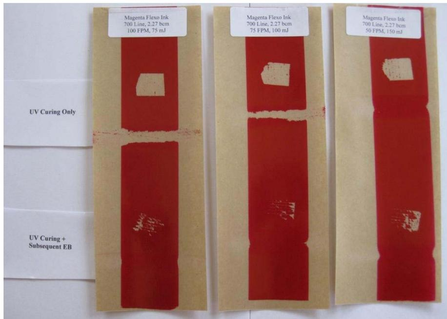
**Figure 3.** Magenta ink samples UV cured at 75, 100, and 150  $\text{mJ}/\text{cm}^2$ . Tape adhesion and MEK resistance is shown before and after subsequent EB exposure.
