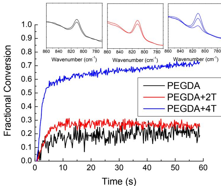
Figure 4. Fractional conversion of acrylate functional groups for three networks under ambient air atmosphere.
