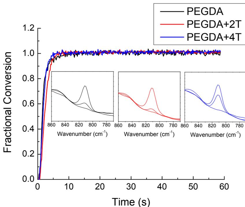
Figure 3. Fractional conversion of acrylate functional groups for three networks under nitrogen atmosphere.
