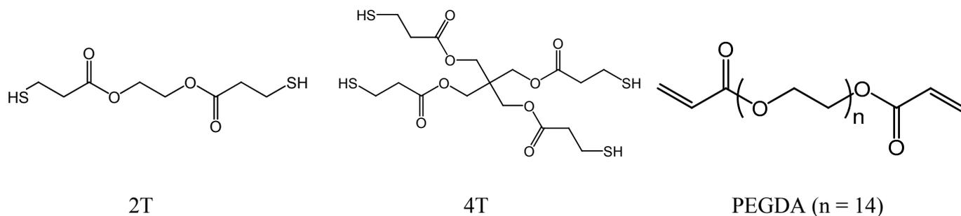
Figure 1. Structures of thiol monomers and acrylate oligomer.
