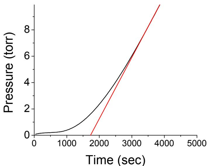
Figure 2. Actual fickian flux curve for CO<sub>2</sub> permeation through a 640 micron PEGDA membrane. Black line is experimental data for permeated gas pressure while red line is the fit to the steady-state slope allowing the calculation of the permeability,  $P$ .
