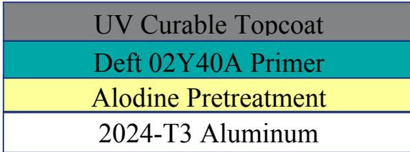
**Figure 2 – Coating stackups diagram**
