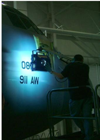
Figure 1 - Curing of stencil coating on C-130
