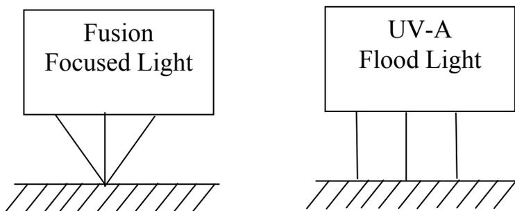
**Figure 3 – Focused versus flood UV lights**
