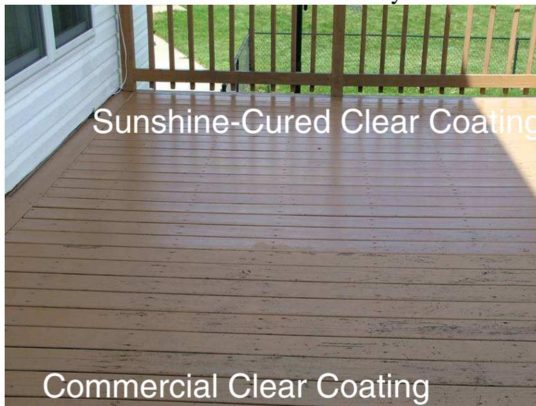
Figure 1 deck after 30 months outdoor exposure in Pittsburgh PA
