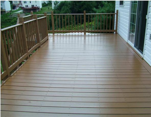
**Figure 8 Field trials basecoat a commercial stain and Sunshine UV PUD clear.**
