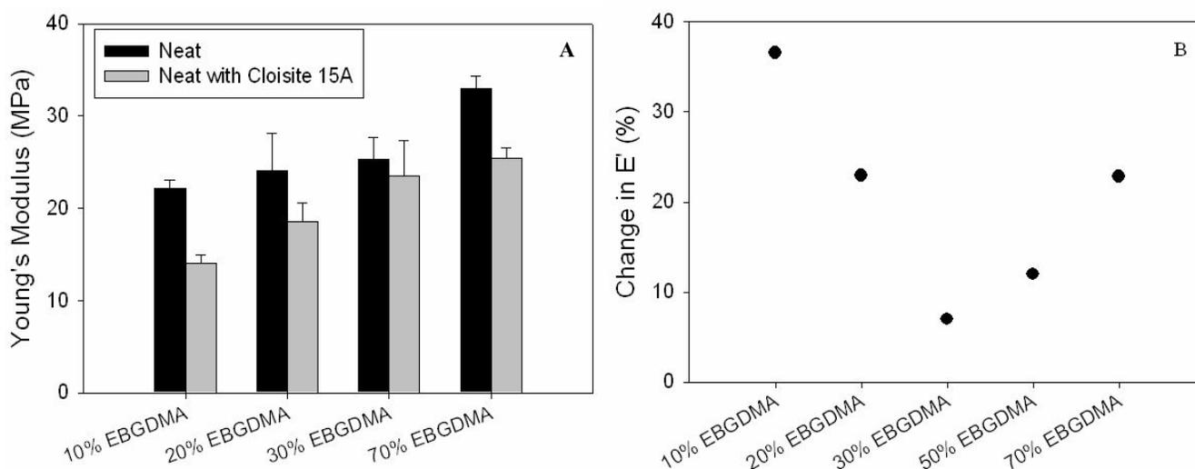
**Figure 4.** (A) Comparison of the Young's modulus of neat versus 3 wt% Cloisite 15A filled thiol-ene polymer with increasing EBGDMA concentration. Neat sample contain 70:30 wt% EBGDMA:PETMP/PEAE (1:1 mol PETMP:PEAE). (B) Percent change in the modulus of Cloisite 15A filled polymer relative to the unfilled polymer as a function of methacrylate concentration.
