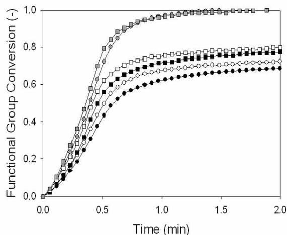
**Figure 5.** RTIR plot of a 10:90wt% mixture of EBGDMA:PETMP/PEAE (1:1mol functional groups) and 3 wt% organoclay. Acrylate (■), ene (□) and thiol (■) conversions for Cloisite 15A samples and conversion of EBGDMA (●), PETMP (●) and PEAE (○) in unfilled samples. Light intensity is 10 mW/cm<sup>2</sup> using 365 nm light.
