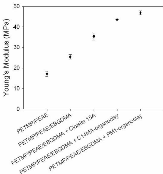
**Figure 2.** Young's modulus of 3 wt% organoclay in 70:30 wt% EBGDMA:PETMP/PEAE (1:1 mol PETMP:PEAE). DMA tests performed at 30°C using a 1 Hz frequency.
