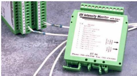
For those plants that desire a more customized solution, the compact sensor and DIN rail transceiver are the building blocks for a completely flexible architecture. The module processes the compact sensor signal and provides a corresponding 0-10 volt analog signal that can be fed to an appropriate PLC or PC control system. Customized screens including password protection, alarm thresholds, data graphing, data export for statistical process control and other features can be designed.
