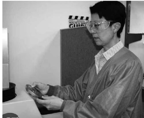
To produce properly cured products, both irradiance and time must be within the prescribed material specification. Like most cooking recipes that require a certain time and temperature, UV recipes usually require minimum irradiance and exposure time (energy density). The common measure of energy density is Joules/cm<sup>2</sup>. (This is a simplification and assumes that you have the right type of UV source for your formulation and that other process parameters are controlled and maintained.)
