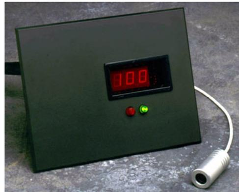
Alternatively, the compact sensor can be installed in the process chamber where it observes the lamp or reflected light. Recall that with online monitoring we are more concerned with relative, minute-to-minute changes in measured UV rather than in the value of the absolute reading itself. This premise allows greater latitude in locating sensors.
