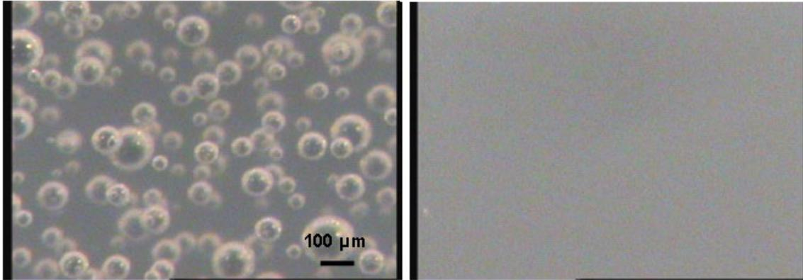
**Figure 2: Deaeration of a radiation-cured coating**
