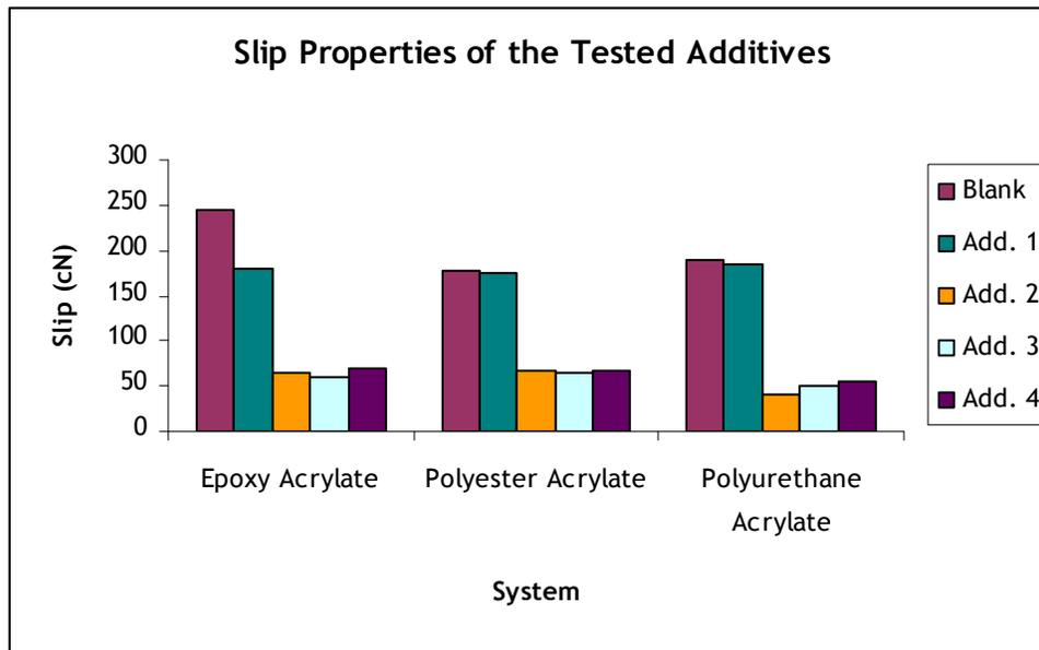
**Figure 3: Slip properties of the tested additives**
