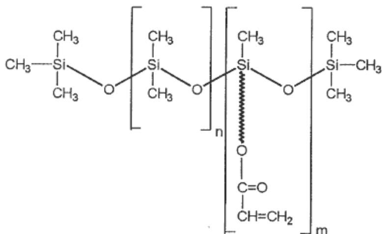
**Figure 1: Structure of organo-modified acrylated siloxane**
