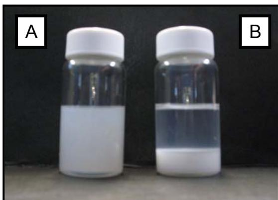
Figure 3. Two vials containing 20 nm aluminum oxide particles dispersed at 1 wt% in a 100% solids UV-curable coating formulation: (A) Stabilized and compatible dispersion, (B) Unstable dispersion showing incompatibility and flocculation of aluminum oxide particles
