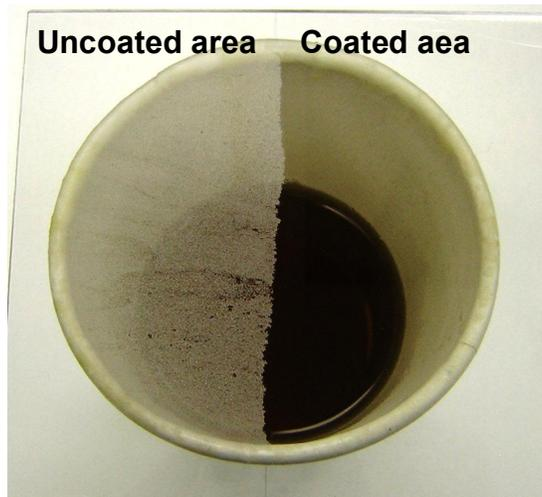
**Figure 2.** Coffee cup fogging test.
