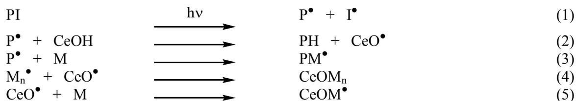
Reaction 1 creates free radicals required for the polymerisation reactions. Reaction 2 is a curing reaction, but reactions 4 and 5 are grafting reactions. Reaction 4 is a grafting reaction of a polymer radical to a cellulose radical and reaction 5 is cure-grafting in which the polymerisation reaction is initiated at the surface of the cellulose. Both grafting reactions are important because they greatly increase the strength of adhesion of the coating to the cellulose.
