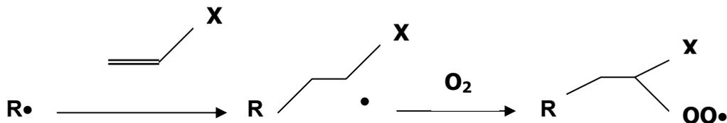
The adverse effects of oxygen inhibition are usually seen at the surface of a coating where the oxygen present in the air/coating boundary layer is able to diffuse into the top layer of the coating. This usually presents as a tacky surface or one with poor scratch or mar resistance. As oxygen inhibition is a surface phenomenon, the problems are usually more evident for thin coatings.
