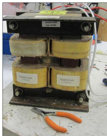
Figure 7b: 2 kW Magnetic Ballast 60 lbs, 500 in<sup>3</sup>
