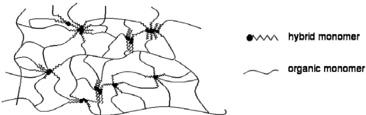
Scheme 2: Organic-inorganic hybrid network formed by the dual UV-curing of an hybrid monomer and organic monomer mixture.
