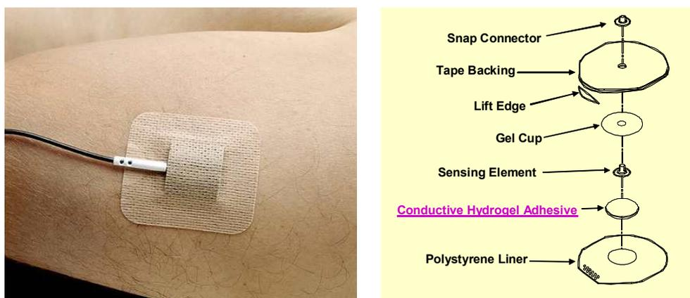
**Figure 1.** Example of a conductive medical hydrogel
