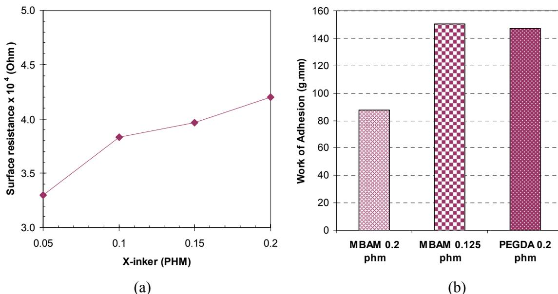
**Figure 4.** (a) Effects of crosslinker on hydrogel resistance. The hydrogels were prepared from AMPS monomer sodium salt and water (50:50) and no glycerol was used. (b) Effect of crosslinker on adhesion. The hydrogel composition was AMPS monomer sodium salt/Water/glycerol = 40:40:20.
