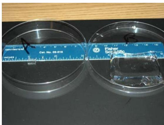
**Figure 2.** Water-swelling of hydrogel with AMPS monomer sodium salt: Water: Glycerol = 40: 40: 20 by wt. (a) Left: before water-swelling ( $\frac{1}{4} \times \frac{1}{4} \text{ in}^2$ ), and (b) Right: a swollen hydrogel after immersed in de-ionized water for 24 hrs ( $1\frac{3}{4} \times 1\frac{3}{4} \text{ in}^2$ )
