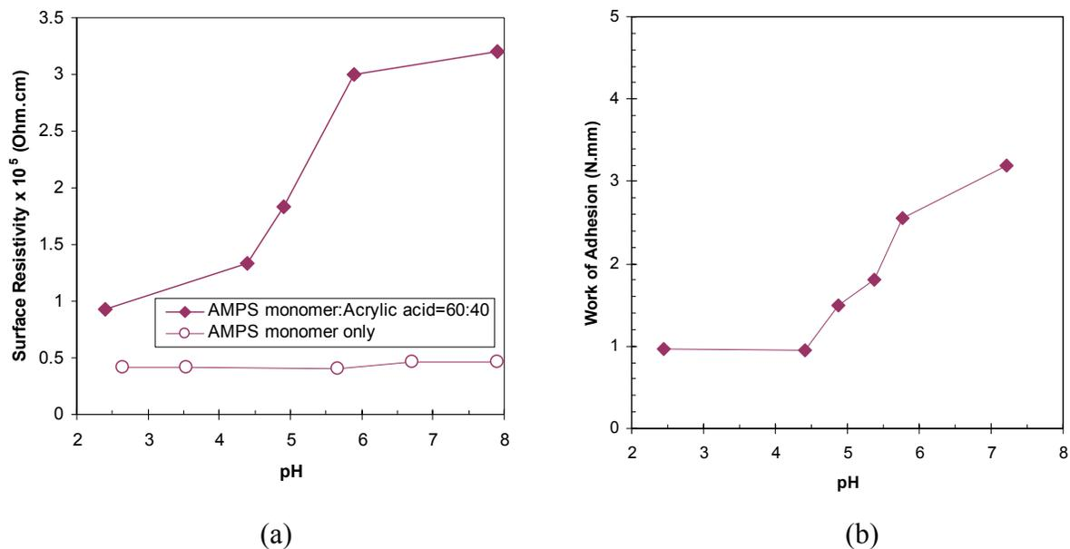
**Figure 6.** (a) Effect of pH content on resistivity (b) Effect of pH on work of adhesion. The crosslinker (MBAM) amount was 0.3 mole % based on total monomers in all cases. The weight ratio of total monomers: water: glycerol was 30: 30: 40.
