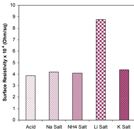
**Figure 7.** Effect of counter ions on the resistivity of hydrogels with AMPS monomer and its salts. The weight ratio of AMPS monomers: water: glycerol was 40: 20: 20.
