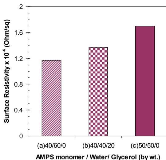
**Figure 3.** Effect of water / glycerol on the resistivity of the hydrogel with AMPS monomer sodium salt
