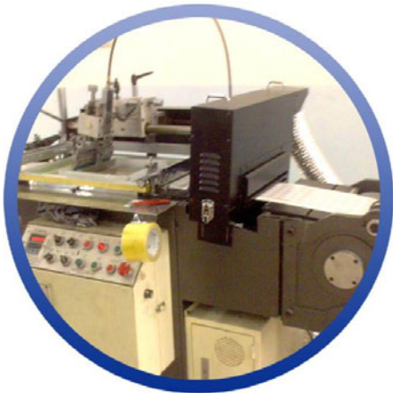
Figure 2 UV attachments for silk screen printing and the products
