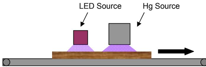
In this configuration, an overall savings in excess of 50% of the energy consumption was realized. Derating the mercury arc lamp also results in increased lifetime of the arc lamp, and better operational stability since arc lamps deteriorate faster as their output power is increased.
