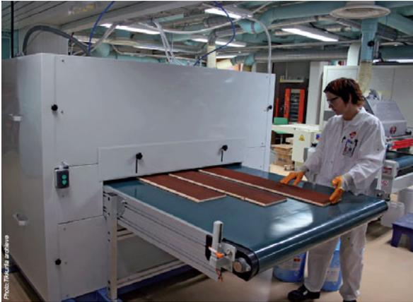
Tikkurila felt that the benefits of solid-state curing are so compelling that adding nitrogen inerting to their process made great sense in the long run.
