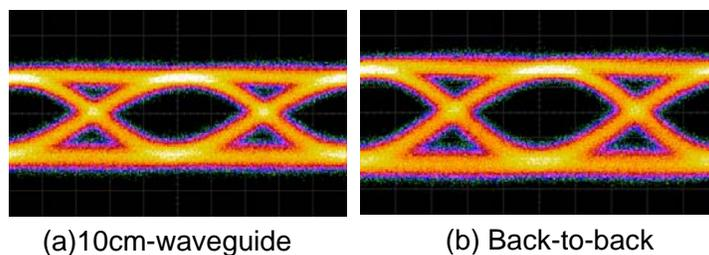
Figure 7 Optical Waveform of 10 Gbits/s transmissions
