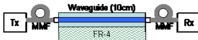
Figure 6 Experimental Setup of 10 Gbits/s transmission
