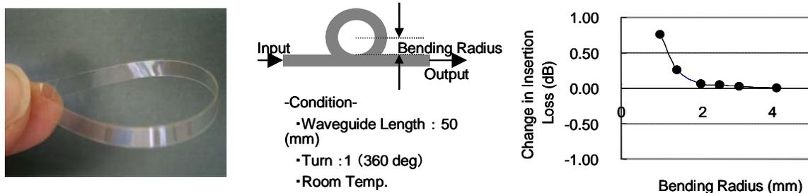
Figure 5 Bending Properties of Flexible Optical Waveguide
