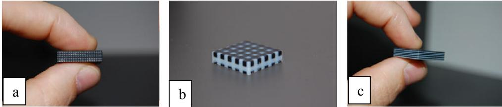
Fig 2: Examples of different types of Digital materials: (a) one material phase is continuous in black and the other one dispersed in white; (b) both phases are continuous; (c) both phases are non continuous.
