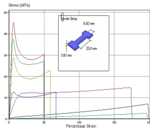
Fig 7: Stress-Strain curves of different *Digital Materials* created from the same parents *Modeling* materials. All these *Digital Materials* were built simultaneously.
