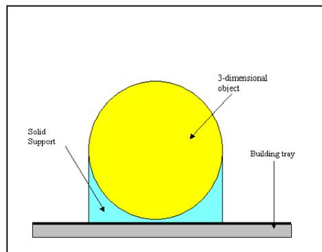
Fig 1: Schematic representation of the result of a *PolyJet Ink Jet 3D Printing* process showing a *3D* model and the solid support construction.
