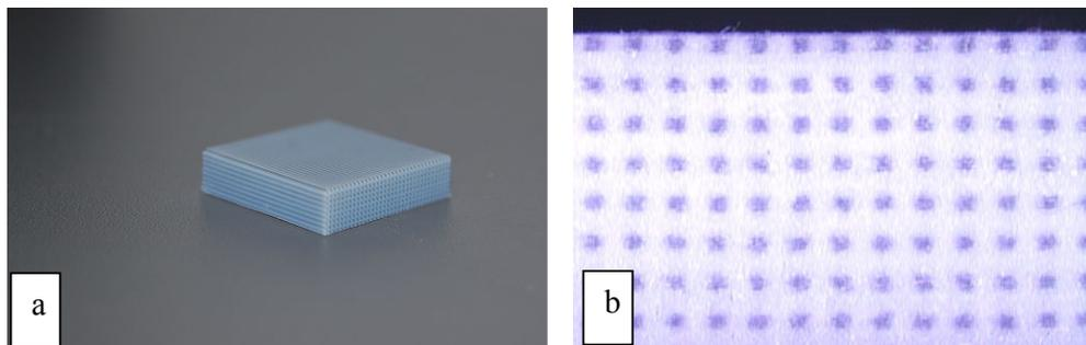
Fig 5: Example of *Digital Material* reinforced by fine "fibers". (a) View showing a *Digital Material* piece; (b) Microscopic view showing 200 micrometer diameter "fibers" cross-section.
