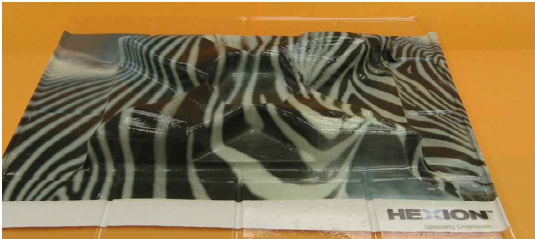
Figure 2. Figure 2 shows an image that was printed flat, cured with UV radiation, laminated, and then post formed with no cracking or loss of opacity.
