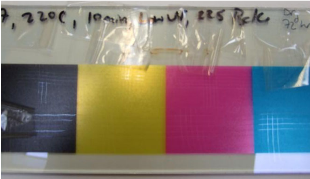
Figure 1. Glass printed with hybrid cure ink, cured with UV, thermally post cured for 10 minutes at 220°C, then soaked in ambient temperature water for 72 hours, tested for crosshatch adhesion immediately afterwards.
