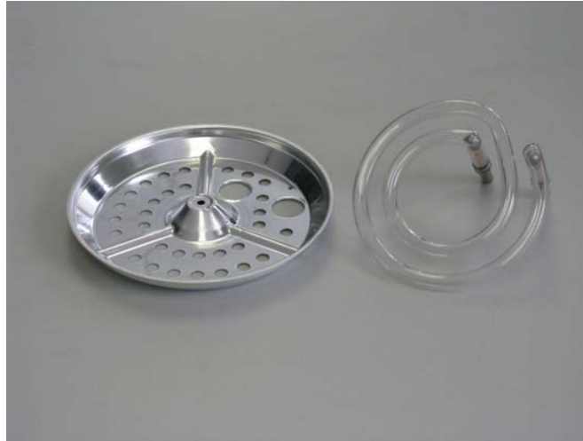
Figure 5: Spiral Lamp and Reflector for Optical Disc Fabrication
