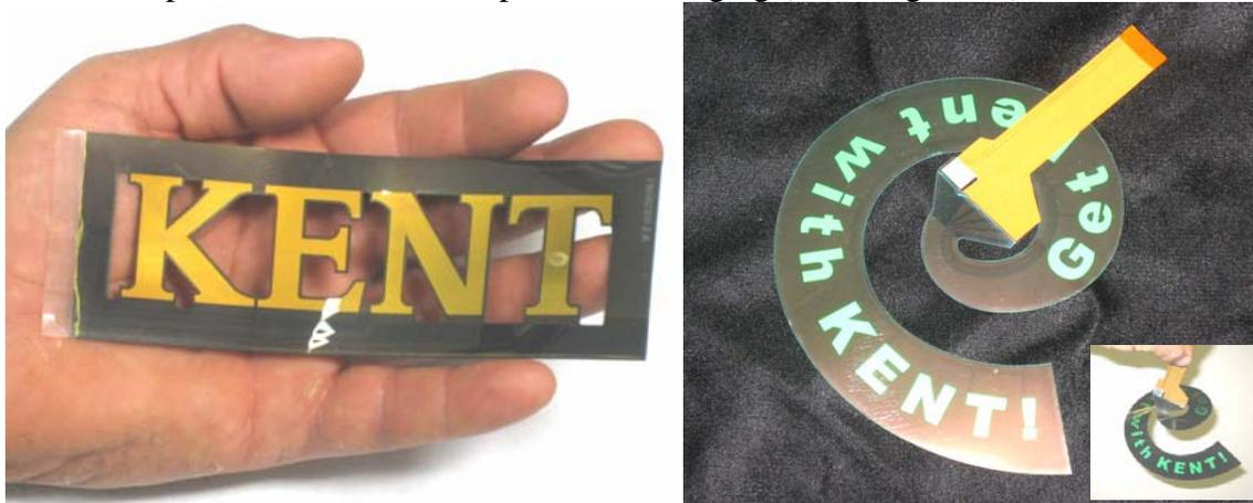
**Figure 11.** Laser edge sealed ITO-based “KENT” display (left) and “spiral” display (right). These demonstrate thru-holes and non-conventional shapes that are not possible with glass displays.
