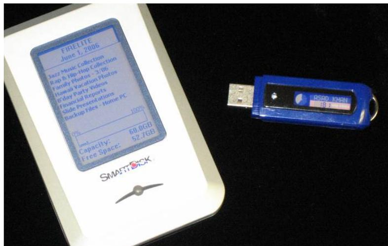
*Figure 1. Glass ChLCDs in USB flash drive (right) and portable hard drive (left) applications.*
