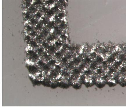
**Figure 4** Mesh Marks on Cured Ag Ink with 75% Ag
