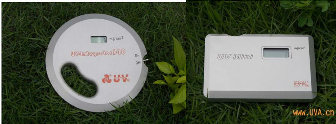
Figure 1. Portable UV energy meters generally employed in industry
