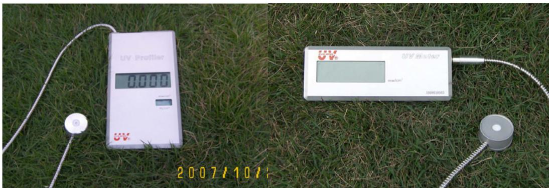
Figure 2. Portable UV radiometers
