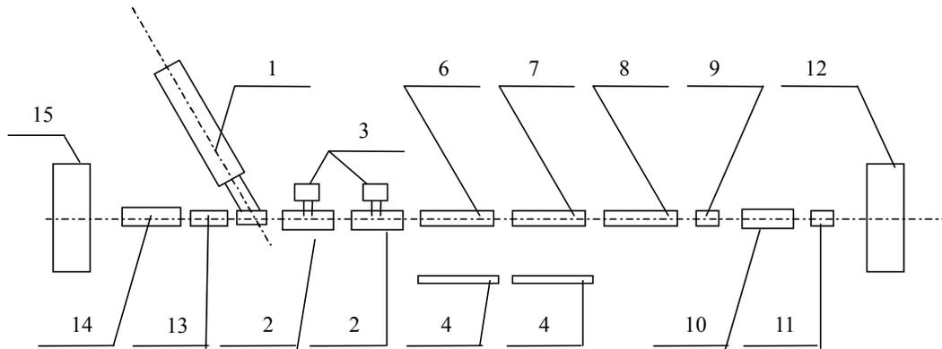
1. extruder; 2. UV irradiation unit; 3. exhaust fan; 4. cabinet of electric controller; 5. cabinet of electrical system; 6. hot water tank; 7. warm water tank; 8. cool water tank; 9. length counter; 10. down-drawing; 11. machine of breakdown; 12. take up; 13. preheater; 14. up-drawing; 15. pay-off.
