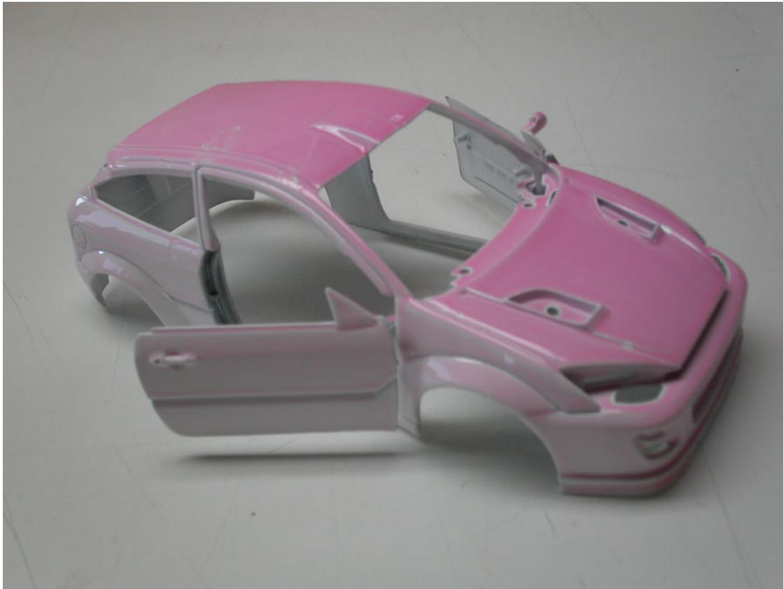
**Figure 3.** Using of the paint-on-photodetector to characterize the UV light exposure of a part with complex geometries.
