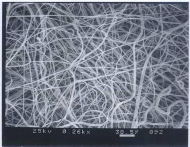
**Figure-2: Non-Woven Polypropylene, Surface Functionalization with no Effect on Breathability**
