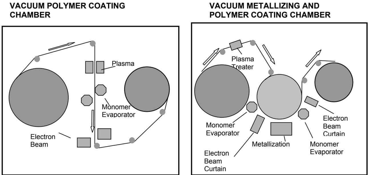
**Figure-1: Polymer Multilayer (PML) Coating Systems**
