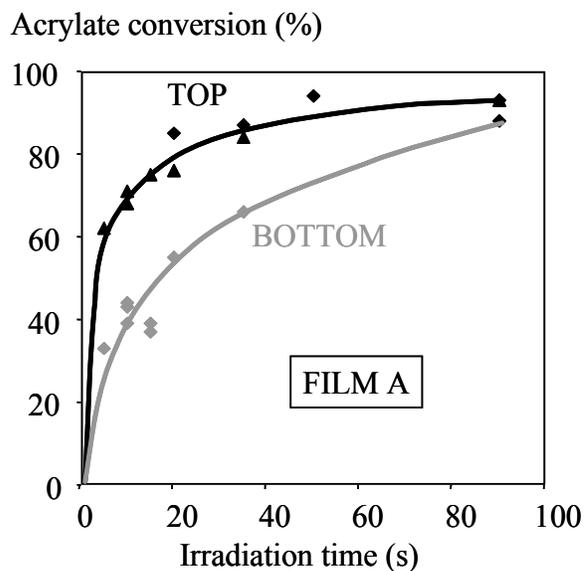
**Figure 8: conversion profile of the top and the bottom layer of film A on plasma exposure 3% BAPO in urethane acrylate, 40  $\mu$ m thick film, room temperature**
