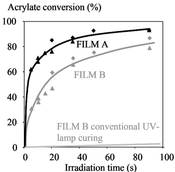
**Figure 7: conversion profile of the top layer of film A and film B on UV-plasma light exposure. Comparison with UV-lamp curing. 3% BAPO in urethane acrylate, 40  $\mu$ m thick film, room temperature**
