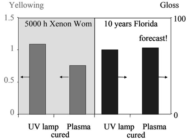
**Figure 12: comparison of the photostability of a plasma- and a UV-cured urethane acrylate**
