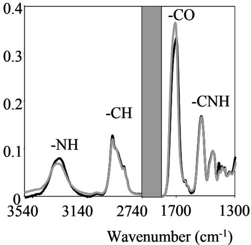
**Figure 11: ATR spectra of the surfaces of a UV-cured and a plasma-cured coating**
