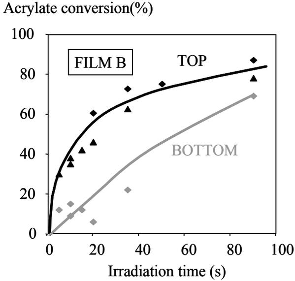
**Figure 9: conversion profile of the top and the bottom layer of film B on plasma exposure**
