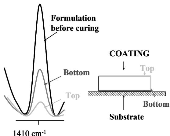
Figure 6: ATR spectra of both sides of the film (top and bottom) after curing and of the formulation before curing as reference
