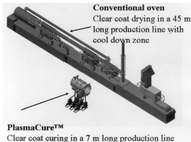
**Figure 14: space requirement of a thermal production line and of a UV-plasma curing installation**
