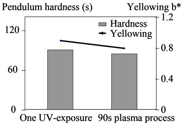
**Figure 13: König hardness and yellowing of UV-cured films irradiated either by a Hg lamp or by plasma process**
