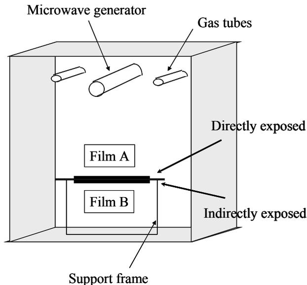
**Scheme 3: experimental setup used in the plasma chamber**
