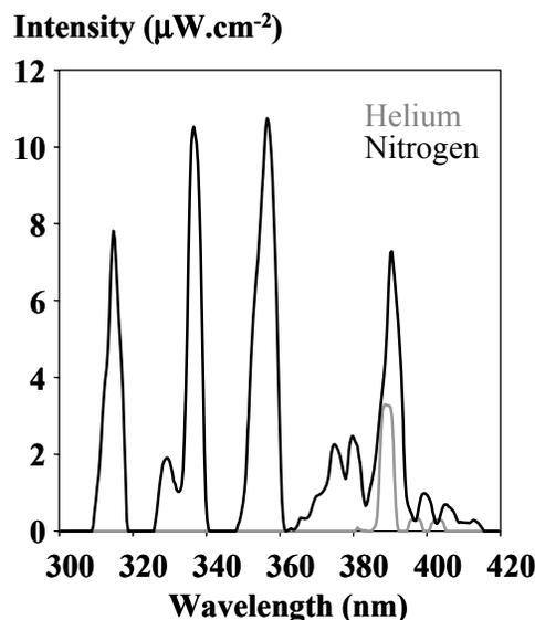
Figure 2: emission spectra of plasma generated by nitrogen and helium
