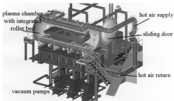
**Figure 15: pilot curing plant**
