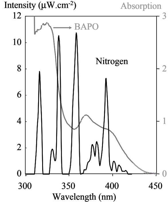
**Figure 10: emission of nitrogen plasma and typical absorption of BAPO photoinitiator**
