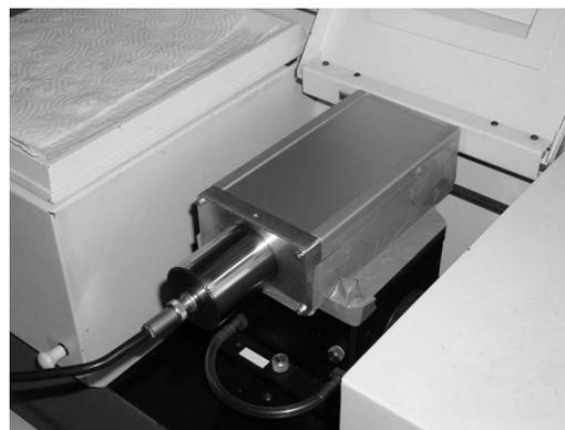
**Figure 5** :  $\text{Xe}_2^*$  excimer lamp attached to the ATR top plate
