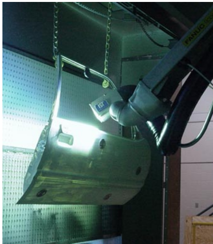
On line robotic UV testing beginning with an automotive door panel outfitted with 10 sensors to measure peak irradiance and dose as the part is moved through the booth
