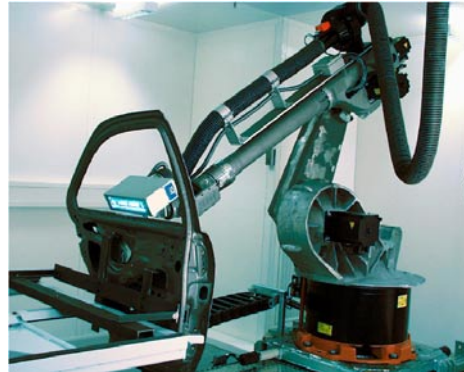
The Daimler-Chrysler UV Technology Center in Ulm, Germany tests robotic cure.
