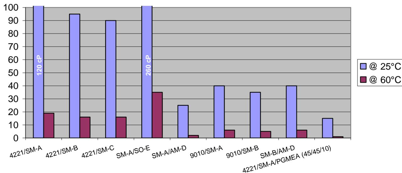
**Figure 1. Viscosity of Resin Blends\***
