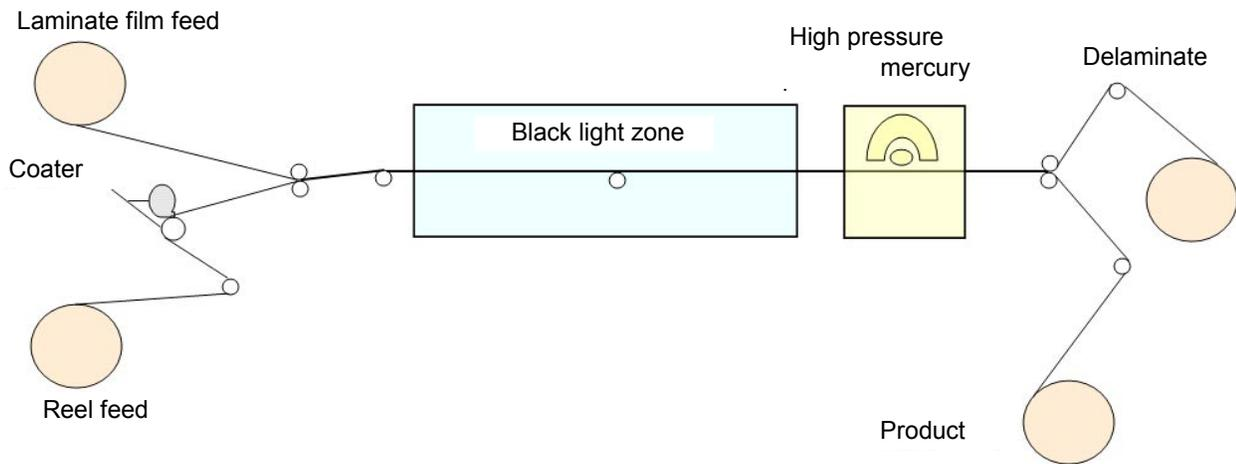
**Figure4.** Coating process scheme
