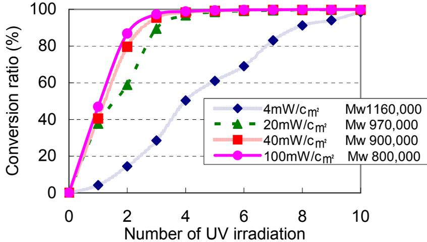
**Figure2.** Correlation between number of UV irradiation and conversion ratio at constant addition of photoinitiator
