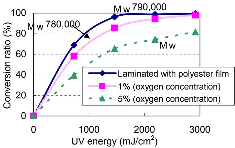
**Figure3.** Influence of oxygen on polymerization behavior
