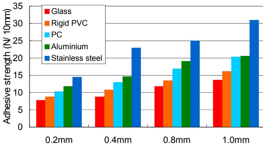
**Figure8.** Adhesive strength of different thickness PSA tape on various adherent materials
