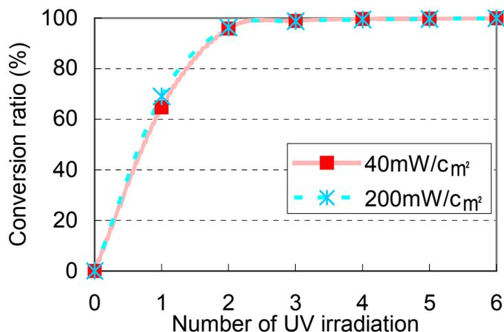
**Figure1.** Conversion ratio change at polymerization where Mw is fixed at 750,000
