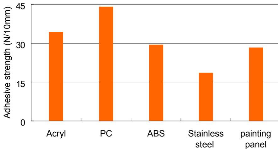
**Figure9.** Adhesive strength of acryl foam double-sided tape
