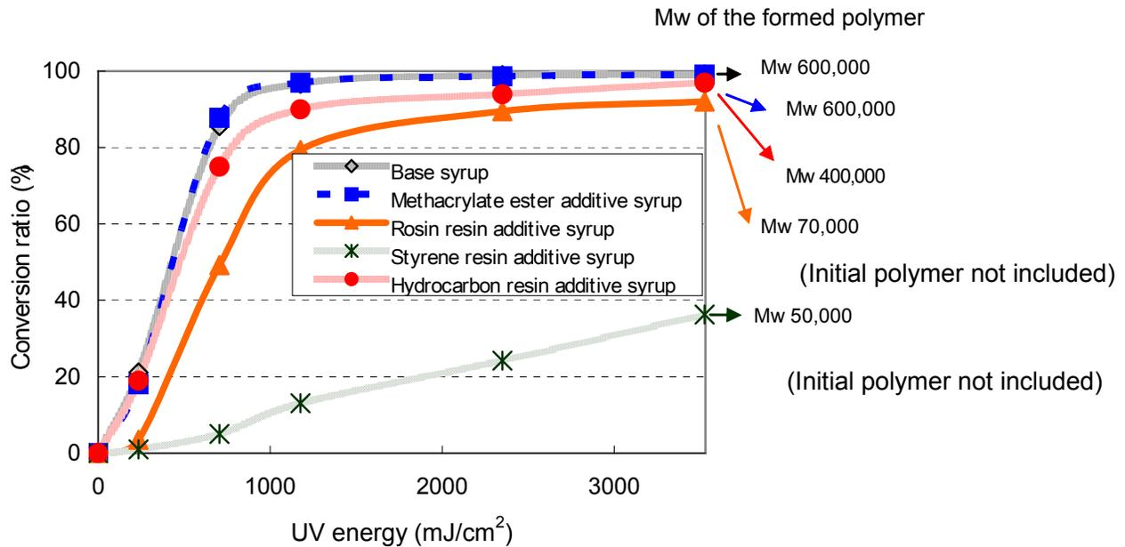
**Figure5.** Polymerization behavior at different tackifier condition
