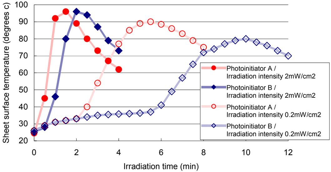
**Figure6.** Polymerization behavior at different absorption coefficient of photoinitiator
