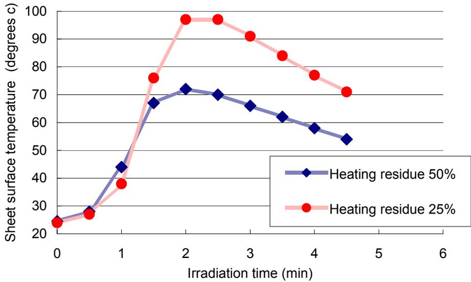
**Figure7.** Heat generation behavior of syrup polymerization at different heating residue
