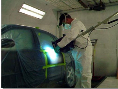
Figure 2: H&S AutoShot 400 UVA lamp used in body shop and lab
