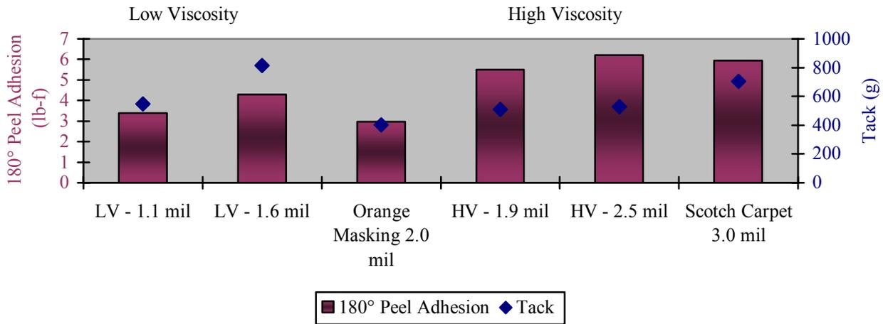
The low viscosity material seems to have a higher peel adhesion and tack than the commercial product being compared with (Orange Masking Tape). The higher viscosity formulated PSA is very strong even at lower adhesive thickness although it is being compared to the Scotch Carpet Tape (3.0 mil adhesive thickness).
