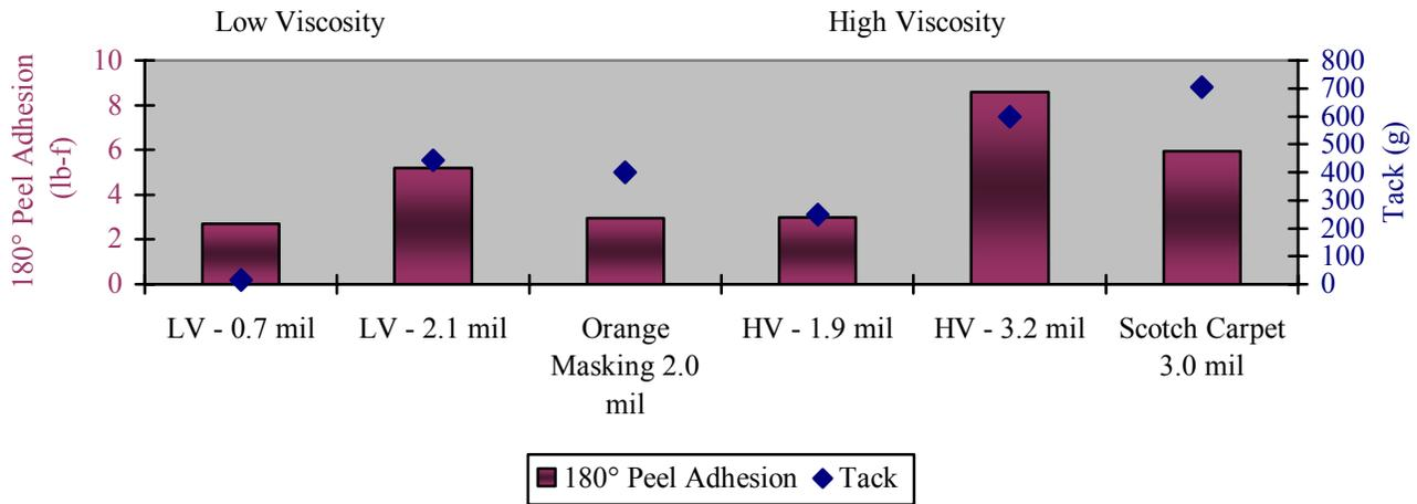
As with most PSAs, when the adhesive thickness is increased, the 180° Peel Adhesion, tack and SAFT are also increased. This is easily seen when comparing the two different application thicknesses for the two formulated UV cured PSAs.
