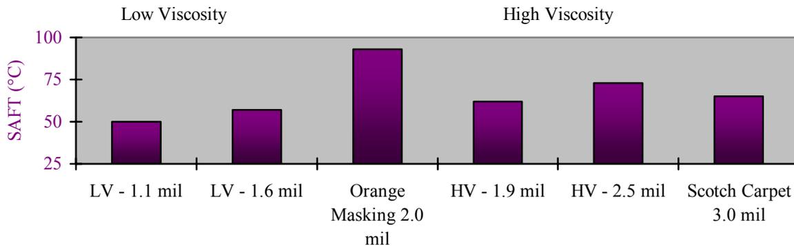
Figure 6 shows the SAFT results. The Orange Masking Tape has a much higher SAFT than any of the formulated UV cured PSAs, but the Scotch Carpet Tape is similar to the UV cured higher viscosity experimental formulations, even though the experimental PSAs are lower in adhesive thickness.
