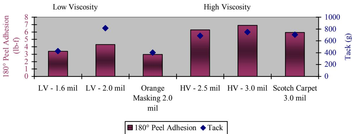
When looking at these formulated PSAs, the performance of the low viscosity #10 rod (1.6 mil adhesive thickness) UV cured PSA is similar to the Orange Masking Tape, but lower adhesive thickness to achieve similar results. A similar trend was seen with the high viscosity formulation, again using the #10 rod to achieve a 2.5 mil adhesive thickness to achieve comparable results to the Scotch Carpet Tape.
