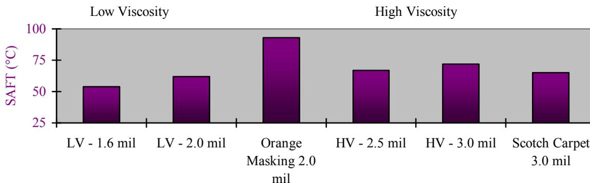
In this set of data shown in Figure 4, the Orange Masking Tape has a higher SAFT than any of the formulated UV cured PSAs. The Scotch Carpet Tape is has a similar SAFT to the two high viscosity experimental formulations.
