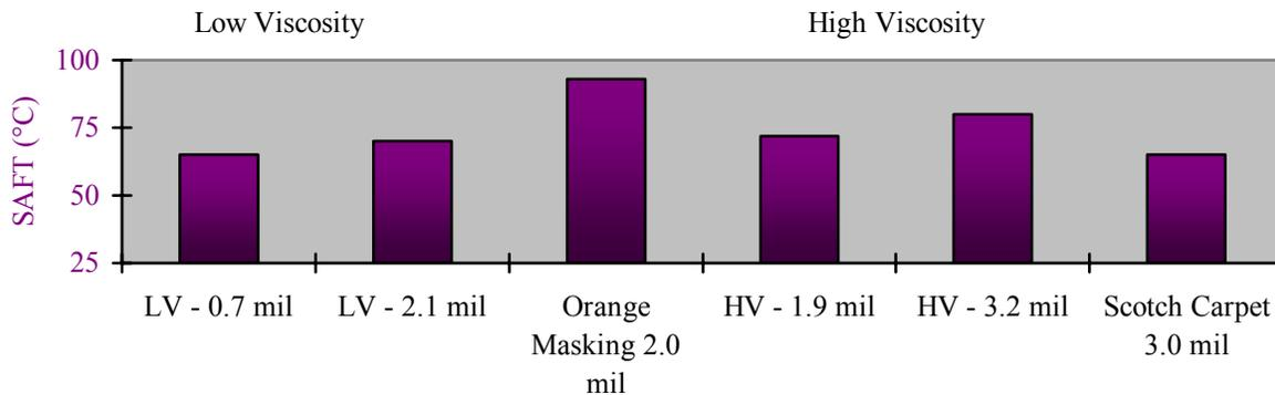
As shown in Figure 2, the adhesive thickness does play a role in the SAFT results. The Orange Masking Tape has a slightly higher SAFT than any of the formulated UV cured PSAs, but the Scotch Carpet Tape is lower than any of the experimental formulations.
