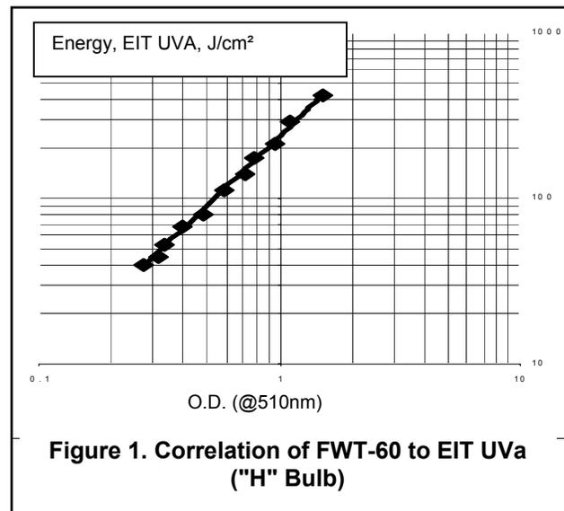
This type of correlation must be done for each specific exposure (type of bulb and spectral distribution). Once done, the correlation can make quick work of multiple measurements.
