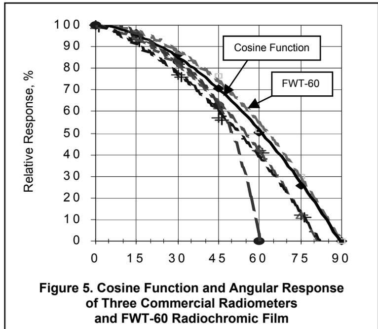
Figure 5. Cosine Function and Angular Response of Three Commercial Radiometers and FWT-60 Radiochromic Film
