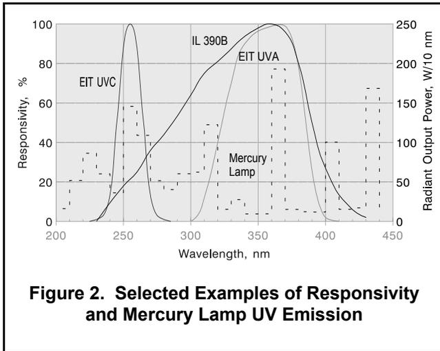
**Figure 2. Selected Examples of Responsivity and Mercury Lamp UV Emission**
