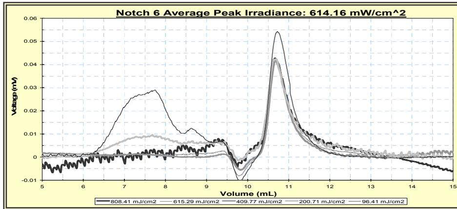
**Figure 12** Combined Chromatograms for All Extractables Made at peak Irradiance 614.16 mW/cm<sup>2</sup>
