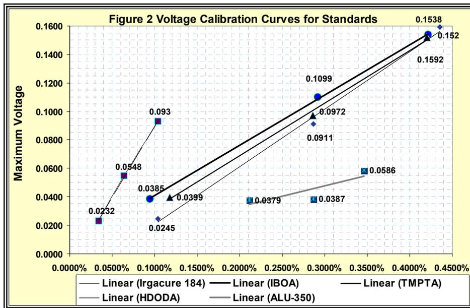
Figure 8 Calibration Curve for All Standard Solutions
