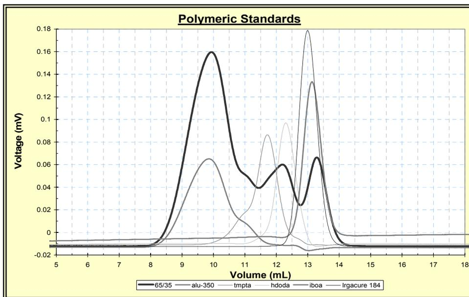
Figure 2 shows the standard solution calibration curves used in this investigation.
