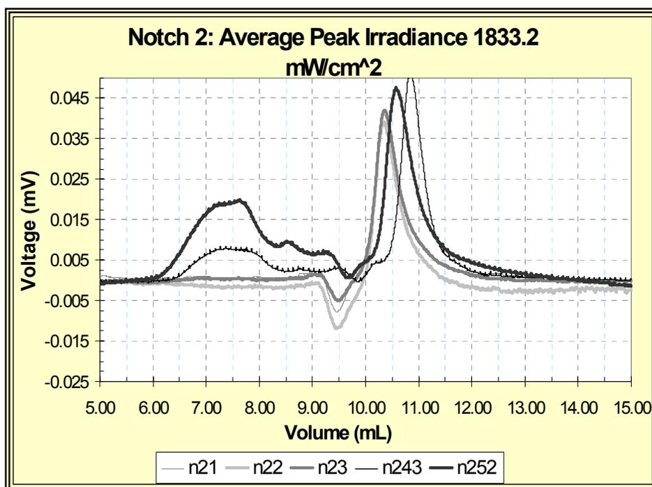
**Figure 9** Combined Chromatograms for All Extractables Made at peak Irradiance 1833.2 mW/cm<sup>2</sup>
