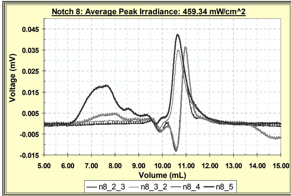
**Figure 13** Combined Chromatograms for All Extractables Made at peak Irradiance 459.34 mW/cm<sup>2</sup>
