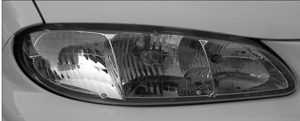
Headlamp Assembly with BMC Reflector and Optically Clear Lens
