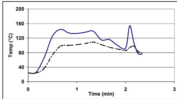
**Figure 2** - Heating / curing profile applied on MDF
