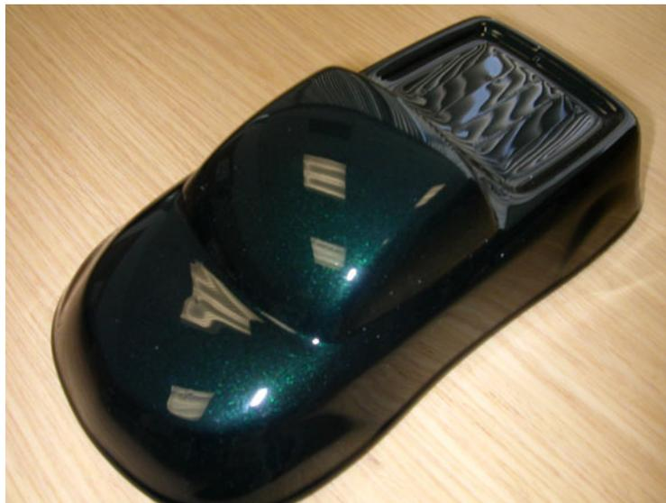
**Figure 8. Photograph of a 3-D Form with a Basecoat/Dual Cure Clearcoat Finish.**
